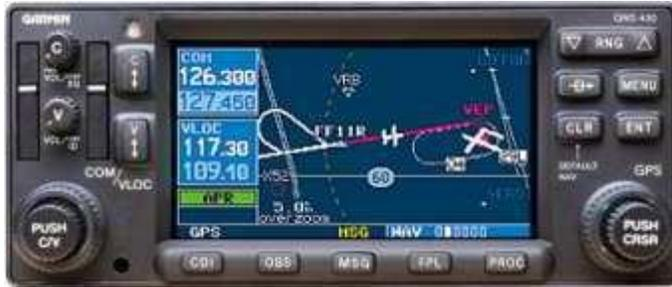
Garmin GNS-430W a WAAS GPS capable of LPV and LNAV/VNAV approaches.
